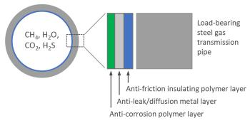
Gas permeation reduction with metal-composite barrier liners.
