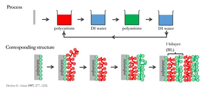
In a typical layer-by-layer (LbL) assembly process, positively and negatively charged components are alternately deposited to produce layered composite membranes.
