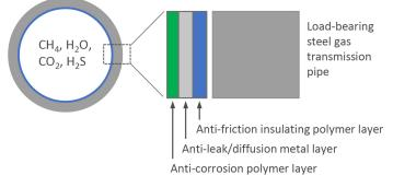
Gas permeation reduction with metal-composite barrier liners.
