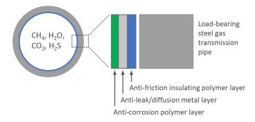
Gas permeation reduction with metal-composite barrier liners.
