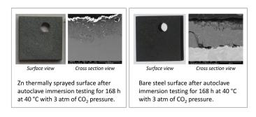
Zn coatings deposition of protective Zn carbonate.
