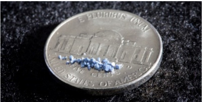
Figure 2. Metal organic framework materials have small porous holes that can selectively adsorb CO 2 over other gases.
