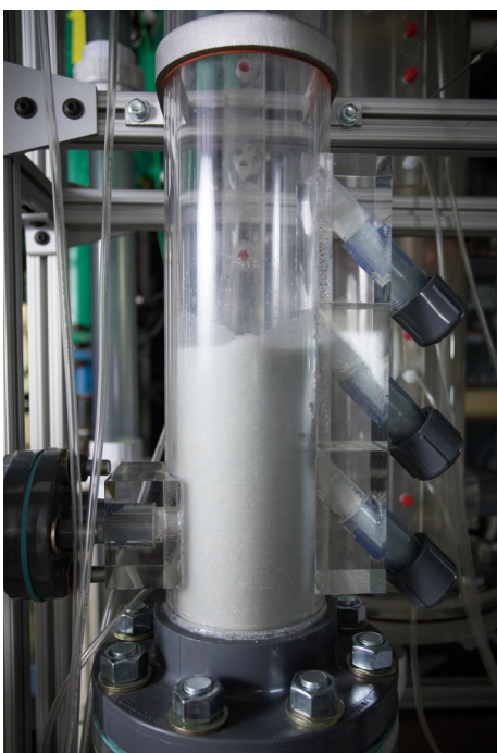
Figure 5. 4-inch diameter cold-flow bubbling fluidized bed.
