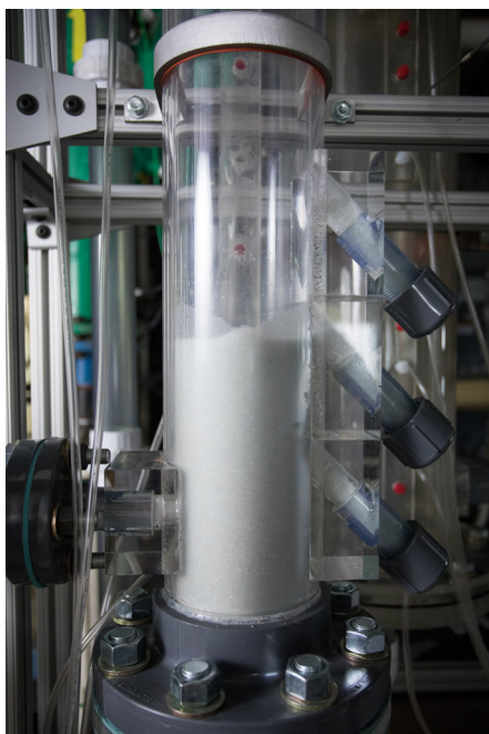
Figure 5. 4-inch diameter cold-flow bubbling fluidized bed.
