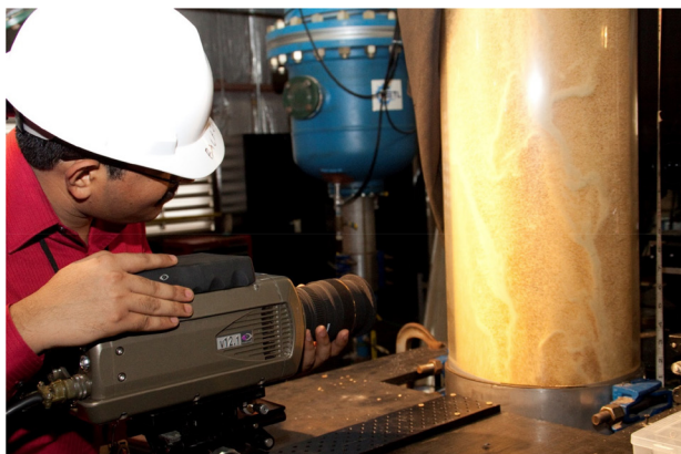
Figure 3. Researcher collecting high-speed video for particle tracking.
