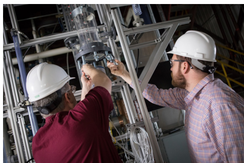
Figure 7. Researchers assembling the cold-flow carbon stripper.
