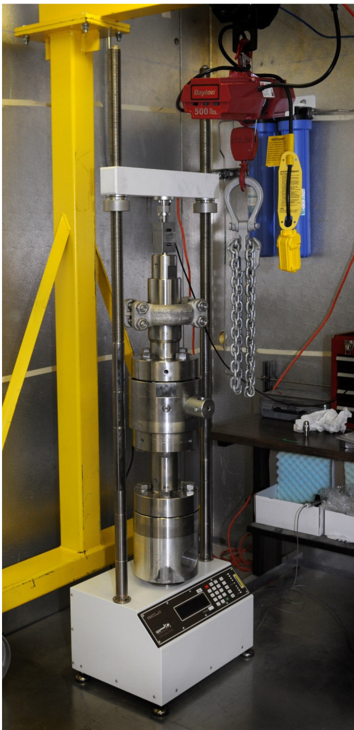
The effective stress chamber (ESC), pictured above, is a critical component of the pressure core characterization and X-ray tool. This chamber is used to measure acoustic, mechanical, and hydraulic properties of pressure core specimens while maintaining in situ pressure and temperature conditions.
