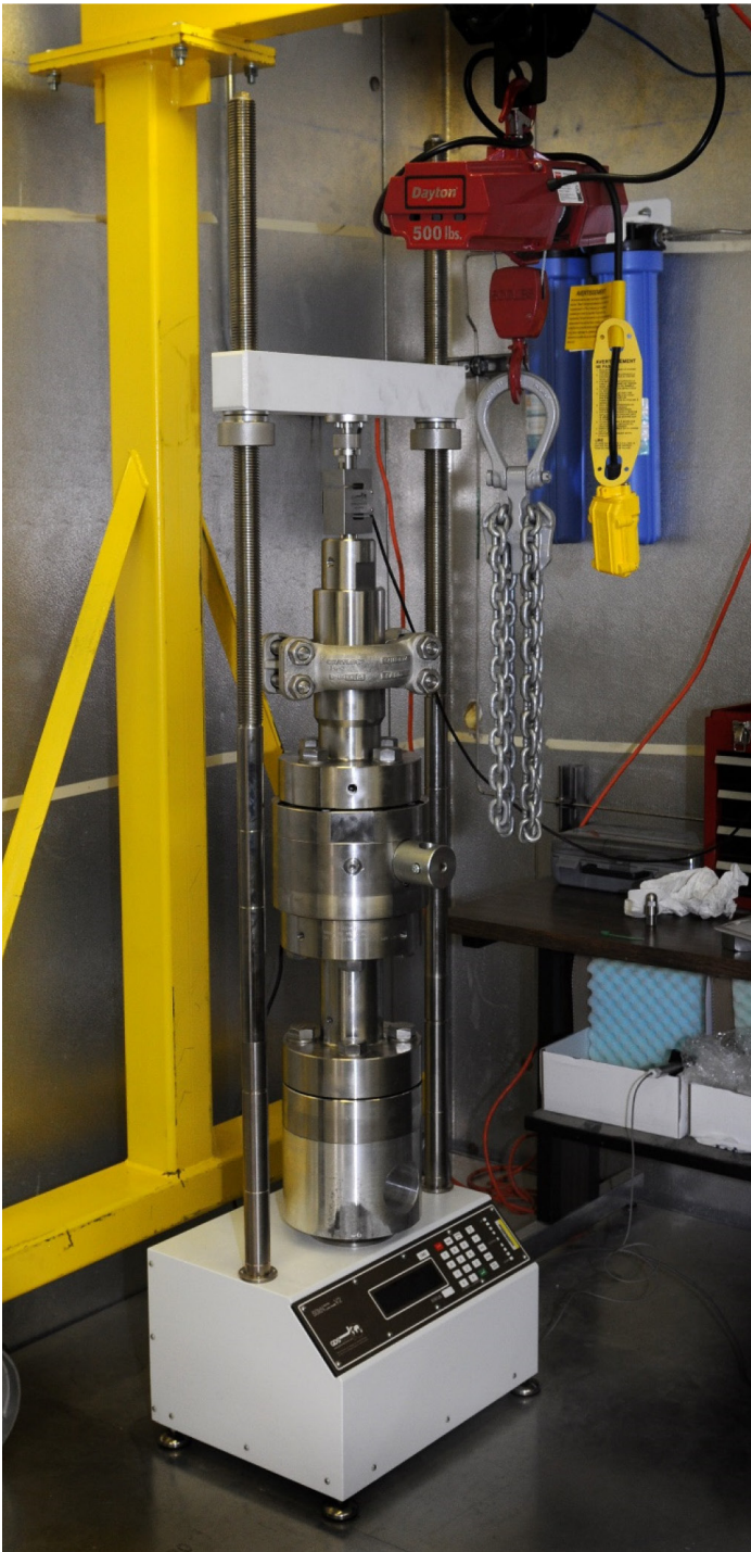
FIGURE 2. The effective stress chamber (ESC), pictured above, is a critical component of the pressure core characterization tools (PCCT). This chamber is used to measure acoustic, mechanical, and hydraulic properties of pressure core specimens while maintaining in situ pressure and temperature conditions.
