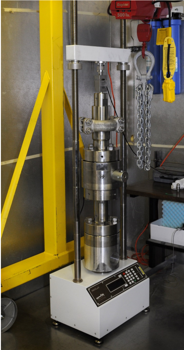
Figure 2. The effective stress chamber (ESC), pictured above, is a critical component of the pressure core characterization tools (PCCT). This chamber is used to measure acoustic, mechanical, and hydraulic properties of pressure core specimens while maintaining in situ pressure and temperature conditions.
