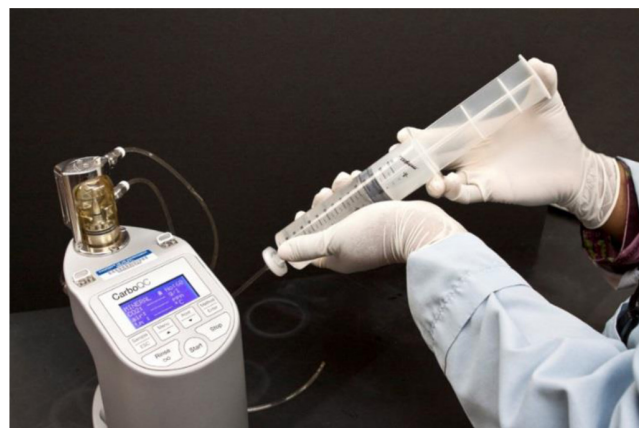
Figure 3: Direct analysis of CO 2 using the volumetric expansion method.
