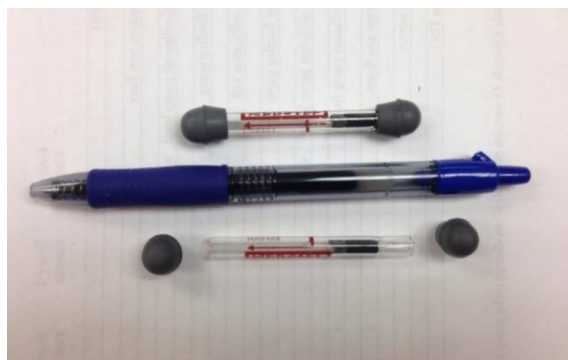
Figure 4. Glass tubes filled with Amborsorb® carbonaceous polymer adsorbent (pen for scale).
