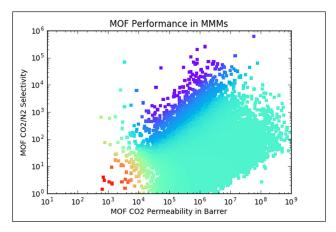
Calculated selectivity versus CO<sub>2</sub> permeability for a large database of MOF materials. Each point is colored based on the relative cost of carbon capture predicted for a hypothetical mixed matrix membrane made using that MOF. Cost is highest for red, moderately high for green, moderately low for blue and low for purple.
