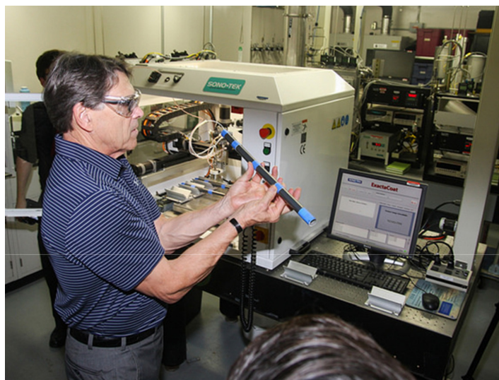
Fig. 6: Secretary of Energy, Rick Perry preparing to insert a commercial fuel cell (Atrix Energy) into NETL's sonic spray coat device for catalyst infiltration.
