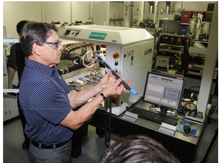
Fig. 6: Secretary of Energy, Rick Perry preparing to insert a commercial fuel cell (Atrex Energy) into NETL's sonic spray coat device for catalyst infiltration.
