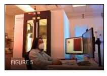
The TESCAN DynaTOM micro-CT scanner is NETL's newest scanner. This system obtains images at the three to tens of micron scale, but is unique in that it has a gantry system and integrated reconstruction
