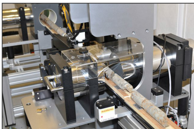
Figure 8. Multi-sensor core logging unit.
