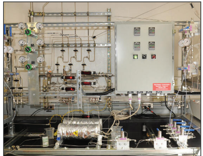
Figure 7. High pressure, high temperature controlled flow through units at NETL.
