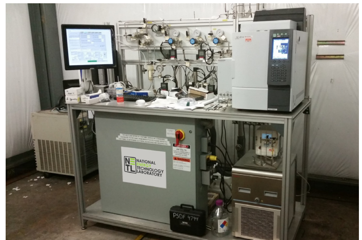
A test apparatus designed and built by NETL to measure gas permeance for CO 2 separation membranes at the National Carbon Capture Center in Wilsonville, Alabama.
