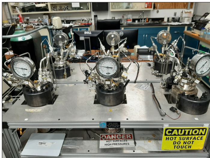
FIGURE 2. Flow-through unit for studying CO 2 -enhanced oil recovery.
