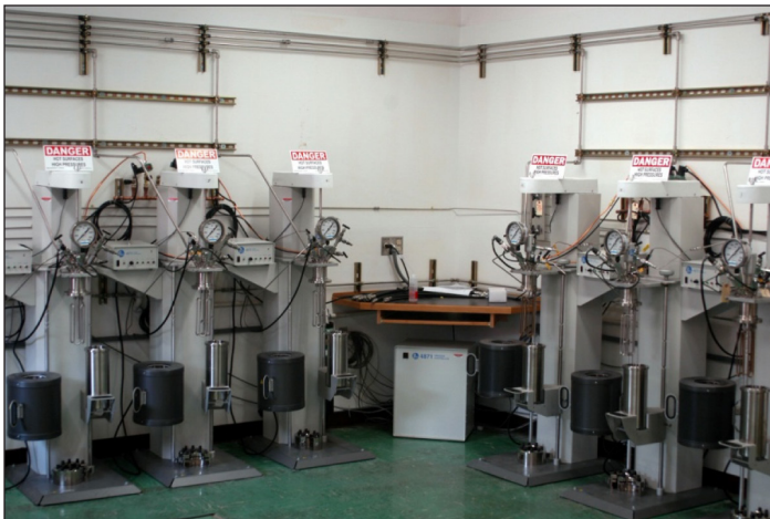
FIGURE 1. Six fixed-head autoclave system with PC interface.
