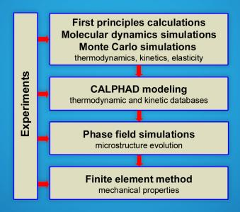
Multi-scale materials simulations supported by critical experiments.
