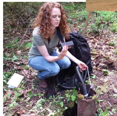
Figure 3. Airborne and ground-based techniques are used in field studies to locate and test legacy wells for methane emissions.
