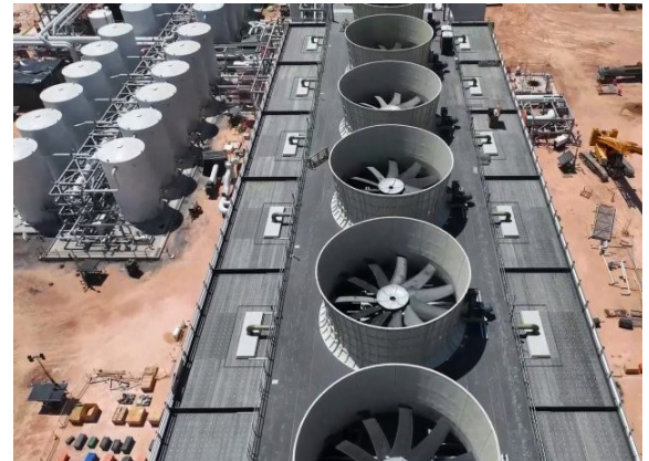
The South Texas DAC Hub will utilize air contactors to draw in air for CO 2 capture. Image: OCED
