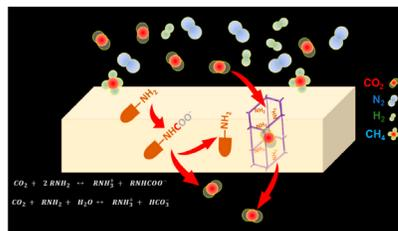
Schematic of CO<sub>2</sub> and amine carrier interaction and an ultrafast CO<sub>2</sub>-selective transport channel inside a facilitated transport membrane.
