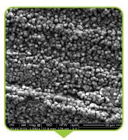
Carbon Steel Surface After Exposure to Corrosive Solvent
