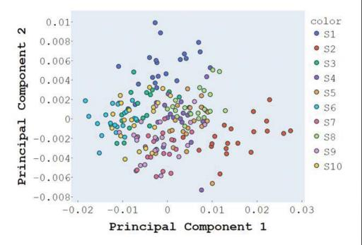
Each Data Point in the Plot Represents One Libs Spectral Data Point of a Corresponding Sample, and Each Sample Has 20 Such Spectra
