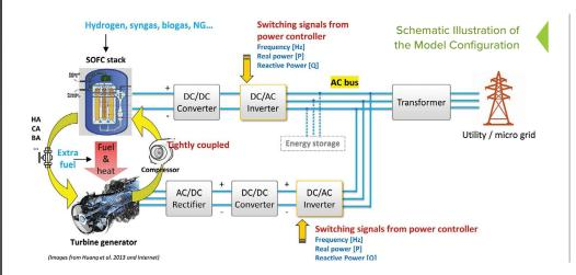
NETL successfully demonstrated that a 50% load change for a solid oxide fuel cell (SOFC) - gas turbine (GT) hybrid power system in less than 10 seconds is possible without violating operability constraints. This rapid transition was accomplished by controlling cathode inlet air flow and temperature to manage temperature gradients in the SOFC.
