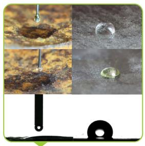
Image of Water Droplet on Untreated Pipeline (Left) vs. DragX<sup>™</sup> Treated Pipeline (Right).
