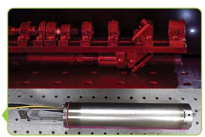
The complete downhole LIBS prototype sensor system was successfully deployed in a test well at the NETL-MGN site at 27-ft well depth (15 ft water depth). Measurements were performed on 14 days over a 20-day period. Results demonstrate the full system works in the target environment without serious complication, which raises the technology readiness level to 5: Lab/bench scale, similar system validation in relevant environment.
