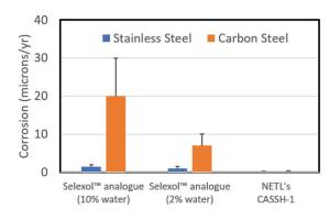
Corrosion Test Results Demonstrated a Notable Decrease in Corrosion Rates Compared to a Benchmark Capture Solvent
