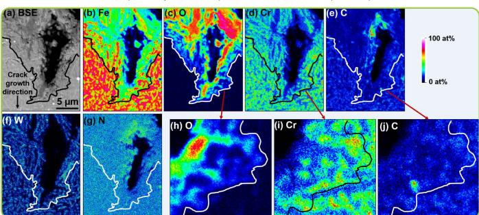
Quantitative Microprobe Analysis of a Crack Tip Near the Fracture Surface for a Specimen Exposed to CO<sub>2</sub>
