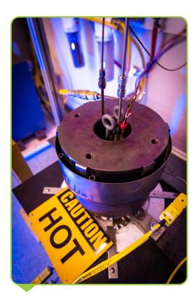
The Autoclave Reactor Is Used to Test Alloys in Flowing sCO<sub>2</sub> at **Extremely High Temperatures and** Pressures to Closely Simulate sCO<sub>2</sub> **Power Cycle Environments**
