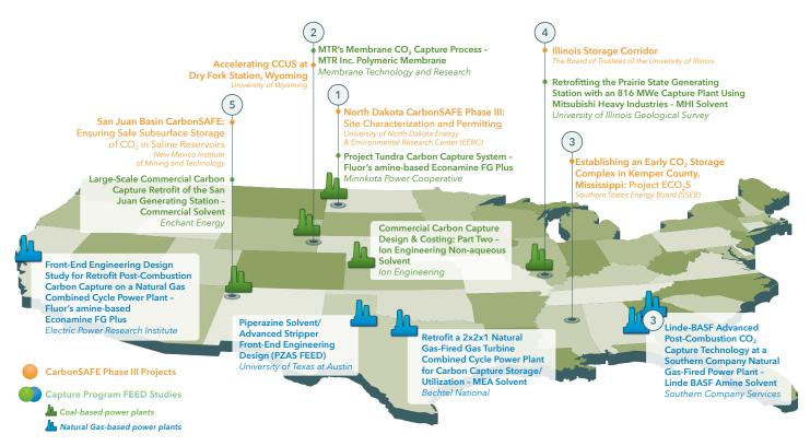
Five CarbonSAFE Phase III projects are aligned with five front-end engineering and design (FEED) studies awarded by DOE's Carbon Capture Program for carbon capture systems on coal and natural gas power plants. These integrated studies show the ability to **supply 50+ million metric tons of CO\_2** for storage per project and evaluate pipeline routes for transport of the  $CO_2$  to the proposed storage complex.
