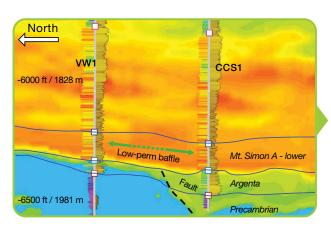
Visualization of **Cross Section Using** Reflection of Seismic **Porosity Inversion**
