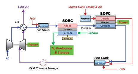
Fuel Cell Technology Integrated with the Grid
