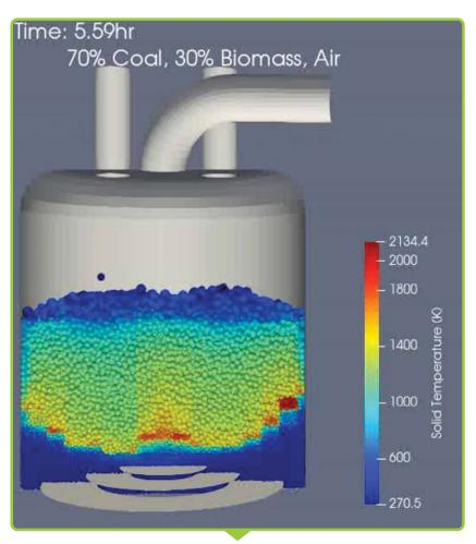
Gasifier Simulations with Mixed Coal-Biomass Feed
