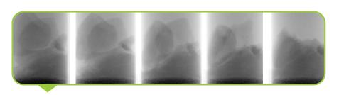
Left to Right: Progressive Degradation of Hydrate Subsamples Over 24-Hr Period, Showing Collapse of Internal Structure In Conventional Systems
