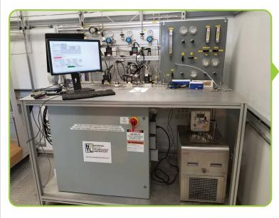
**NETL's Membrane** Test Unit at NCCC for Coal Flue Gas Decarbonization (Operational)
