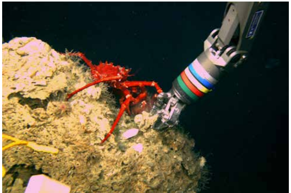
Figure 3. The mechanical arm of the Global Explorer ROV samples methane-derived authigenic carbonate near a seep site on the Virginia margin. The British Geological Survey will conduct uranium-thorium geochronologic analyses on the rocks to determine the timing of methane emissions. Image acquired by Oceaneering, Inc.
