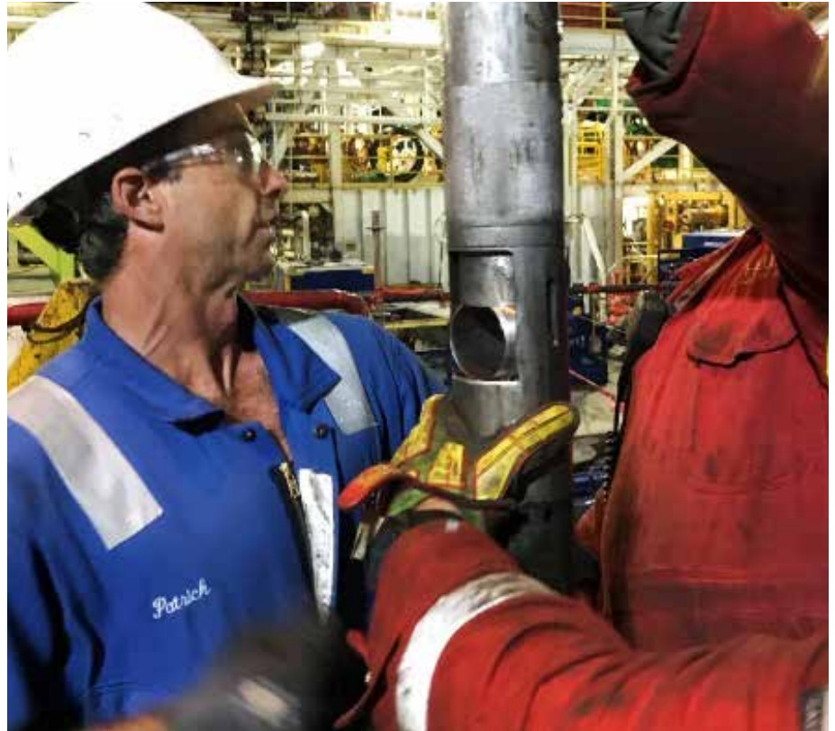
Figure 3. Patrick Riley of Geotek inspects a successful PCTB deployment (note the closed position of the ball valve) on the deck of the Q4000.
