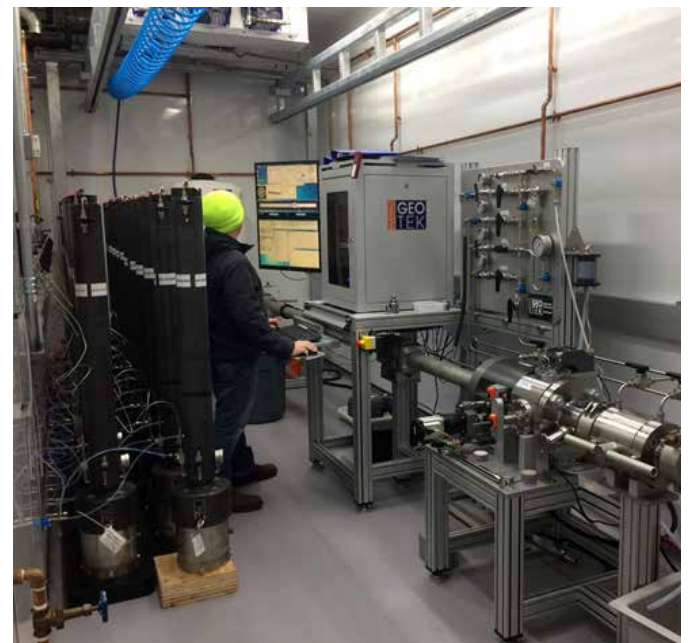
Figure 6. Lab manager Josh O'Connell examining UT-GOM 2 -1 pressure cores with the mini-PCATS at the UT Austin pressure core lab.
