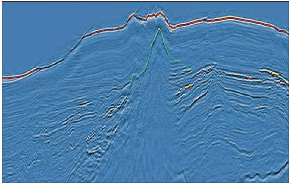
**2C)** a High-relief “BSR” (denoted by green line) which is not bottom-simulating and represents locations where the BGHS is perturbed by local variations in heat flow. Data courtesy of WesternGeco.
