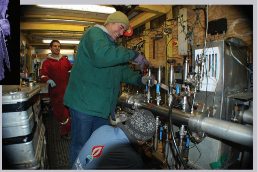
**Figure 4:** Carlos Santamarina and Tae Sup Yun making measurements on a pressure core using the IPTC.
