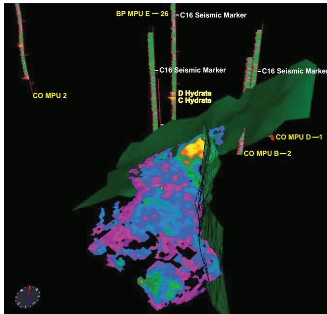
**Figure 2:** Milne Point—Mount Elbert gas hydrate prospect. Three-dimensional image of a fault-bounded, high amplitude feature (in a palette of colors ranging from yellow to magenta; the yellow-imaged portion of the structure contains the thickest and most concentrated gas hydrate). Also shown are the bounding faults (in green) and gas hydrate occurrences in nearby well penetrations. The well penetrations show downhole-measured geophysical data indicative of gas hydrate occurrence (in yellow).
