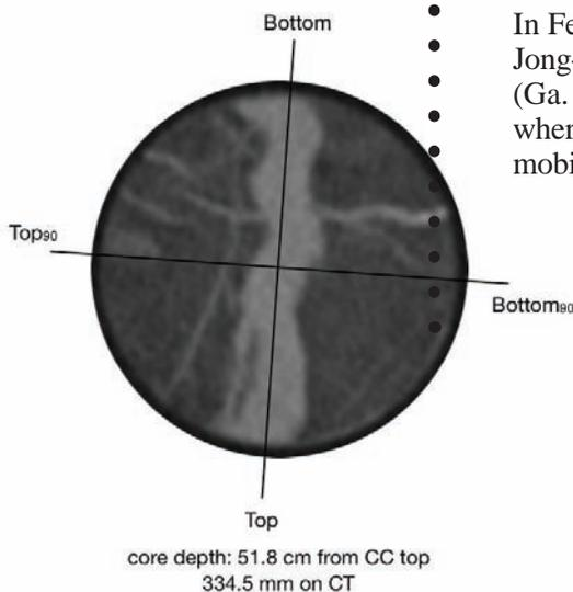
**Figure 2:** Horizontal slice through one of the pressure cores showing two locations where IPTC measurements were made. Hydrate veins are white; clay sediments are dark.
