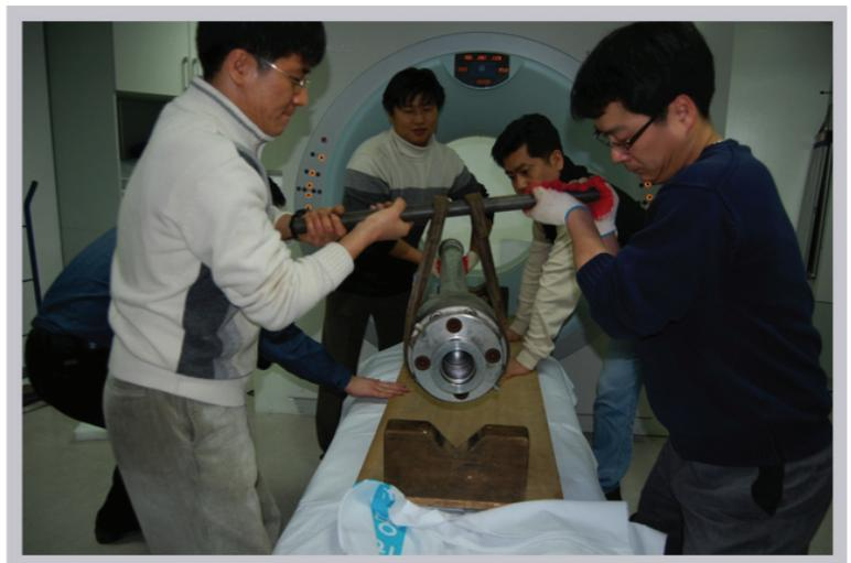
**Figure 1:** Scientists from KIGAM load a pressure core in a storage chamber onto the bed of the X-ray CT machine in Daejeon, Korea.
