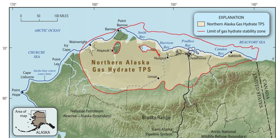
Figure 1: Map showing the Northern Alaska Gas Hydrate Total Petroleum System (TPS) (shaded in tan), and the limit of gas hydrate stability zone in northern Alaska (red outline).
