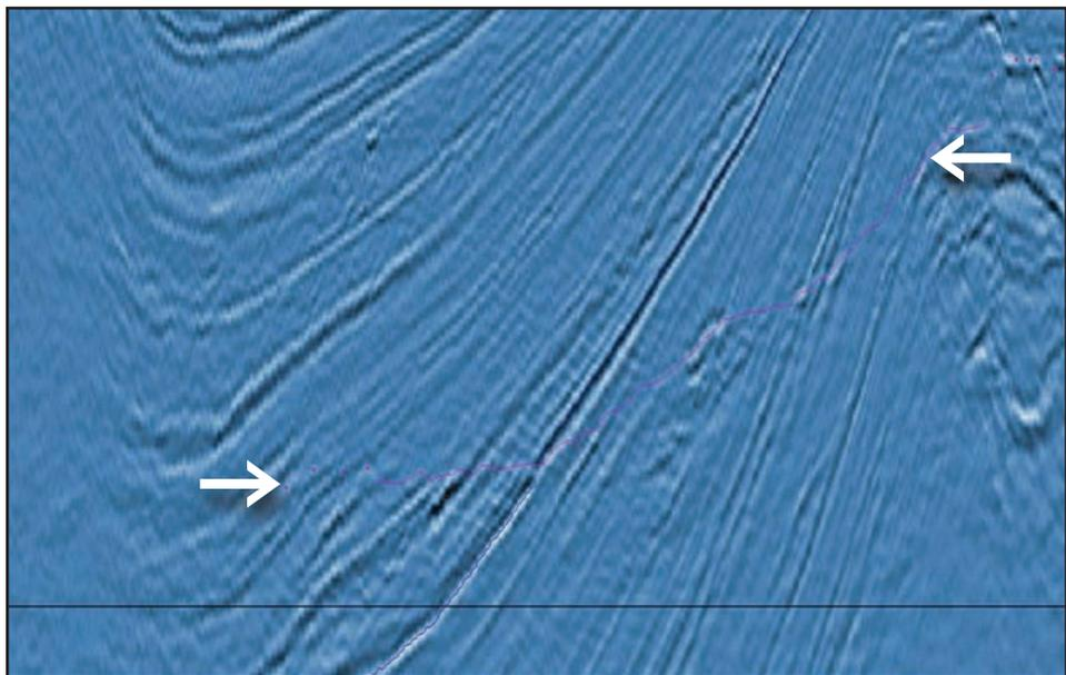
**2B)** a Segmented "BSR" formed by the alignment along a sea-floor simulating horizon of anomalous seismic events including bright spots, terminations, and phase reversals. Data courtesy of WesternGeco.
