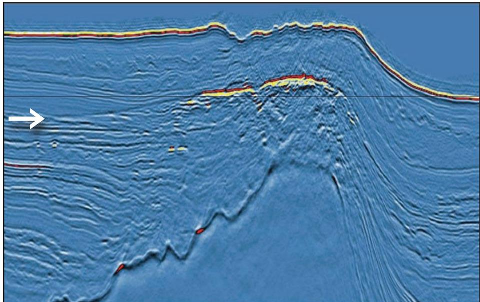
**2A)** a Continuous BSR with polarity opposite the seafloor and clear cross-cutting relationship to strata. Data courtesy of WesternGeco.
