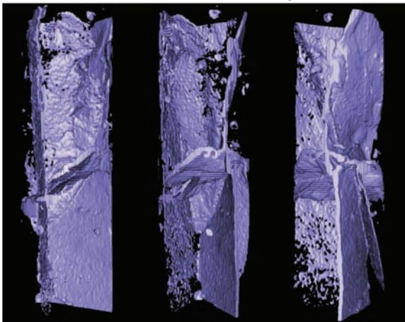
**Figure 3:** A three-dimensional reconstruction of a short section of core. Sediment is transparent, gas hydrate is blue. Hydrate veins in the pressure cores were generally subvertical, but at varied orientations.
