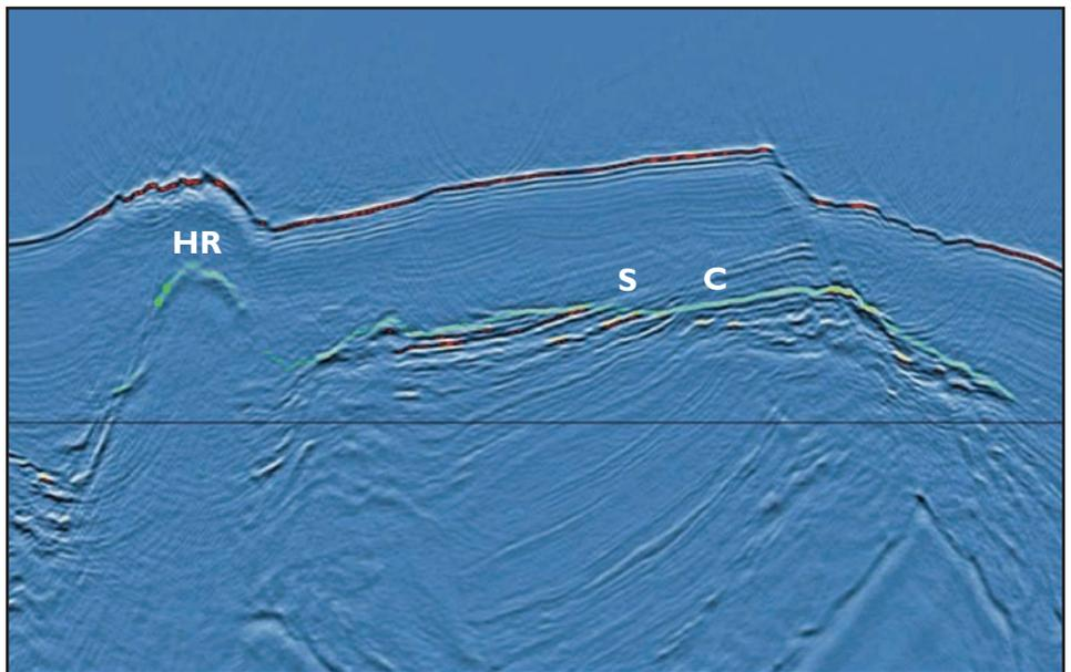
**2D)** a example where the BGHS shown a combination of High-relief (HR), segmented (S) and continuous (C) morphologies. Data courtesy of WesternGeco.
