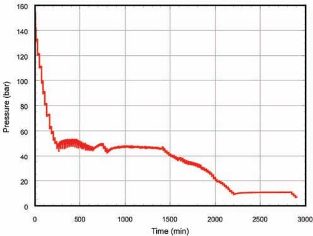
**Figure 5:** Depressurization curve for a core showing extended pressure “plateau” at hydrate stability boundary.
