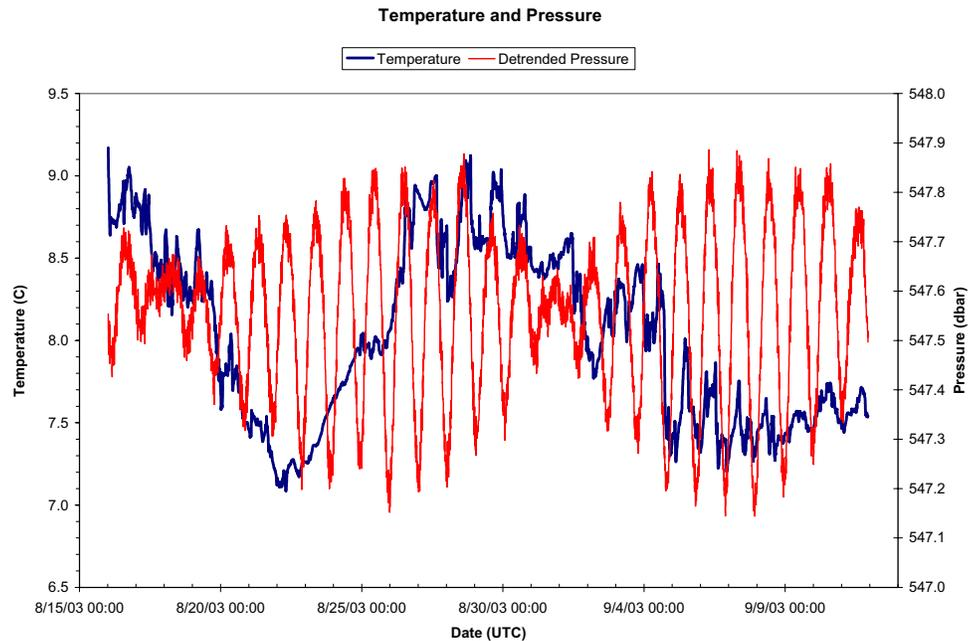
*Data from the CTD show a typical variation in temperature over a range of almost 5°F (3°C) and smaller diurnal cycles are evident. The pressure data (the first such data series recorded from Bush Hill) show clear lunar cycles in tides that correlate well with temperature cycles*
