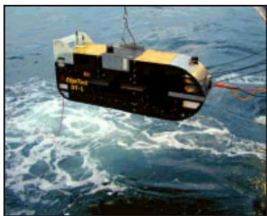
Deep-Towed Side-Scan Sonar and Sub-Bottom Profiler
