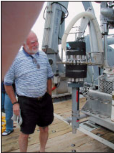
Dr. Bob Woolsey admires the FSU/UNC in-situ pressurized pore-water sampler.
