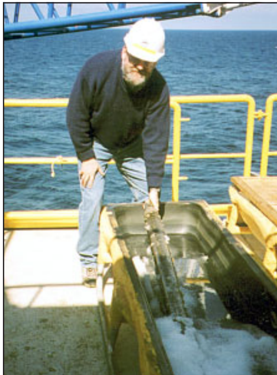
Dr. Frank Rack, Assistant Director of the Ocean Drilling Program and Staff Scientist, during Leg 204 of the Ocean Drilling Program, handles the ODP Pressure Core Sampler on the deck of the R/V JOIDES Resolution. It contains gas hydrates in an ice bath awaiting controlled degassing in the lab.
