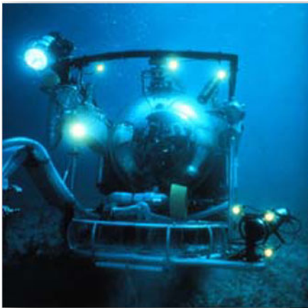
The four-person submersible, Johnson Sea Link II and an improved hydrate drill were used to recover gas hydrate in the northern Gulf of Mexico.
