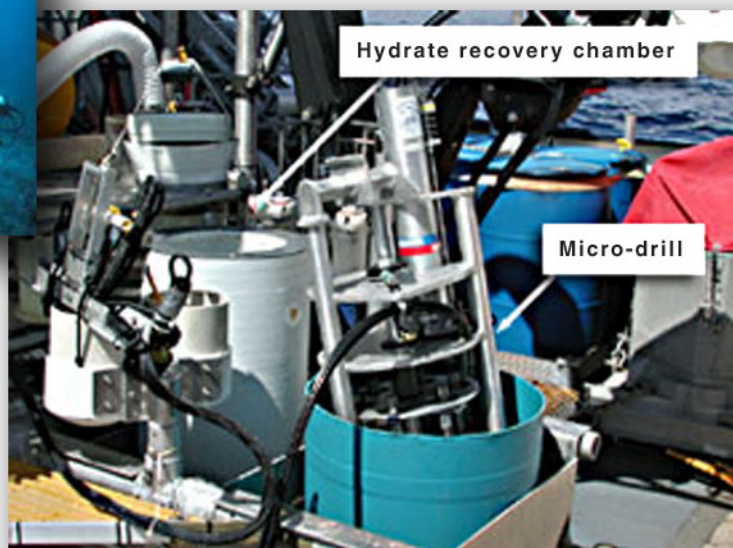
The four-person submersible, Johnson Sea Link II and an improved hydrate drill were used to recover gas hydrate in the northern Gulf of Mexico.
