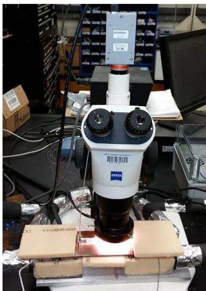
**Figure 11: Imaging system and chip on TTP.**
