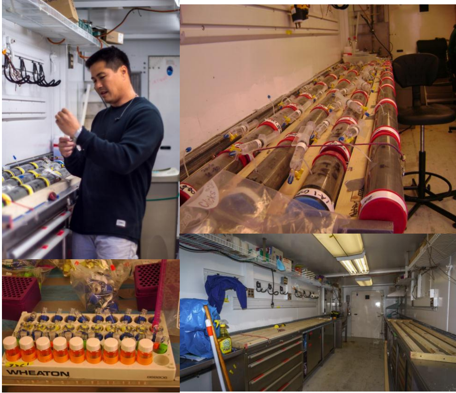
Figure 6: Pore water sampling using Rhizon samplers and distribution of samples.
