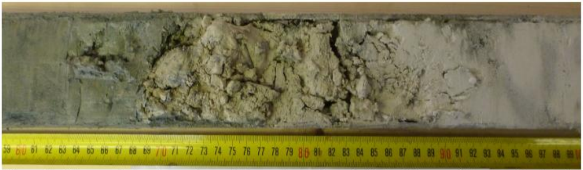
Figure 2: The transition from glauconitic sandy-mud to chalk in 70 cm subbottom depth. The indurated part forms a depositional hiatus.
