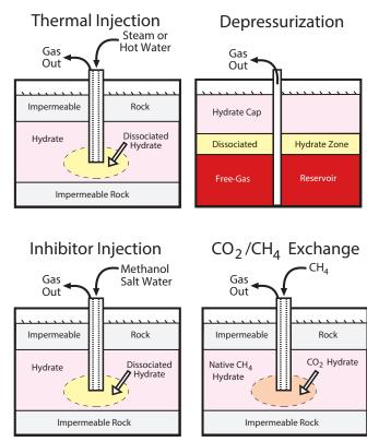
*Figure 8. Schematic of proposed methane hydrate production methods.*
