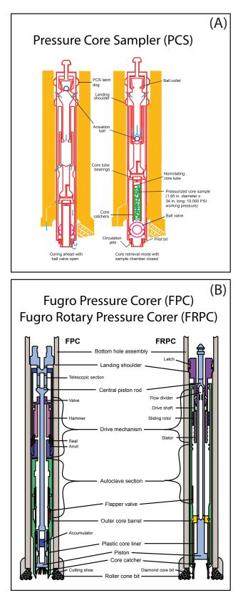
Figure 14. Diagrams of pressure core systems: (A) Pressure Core Sampler (PCS); (B) Fugro Pressure Corer (FPC) and Fugro Rotary Pressure Corer (FRPC).
