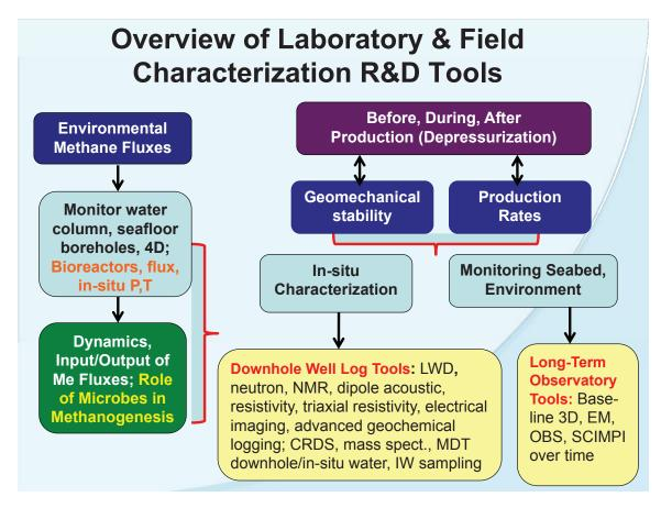
*Figure 16. Overview of laboratory and field tools used to characterize the occurrence of methane hydrates associated production and carbon cycle issues.*
