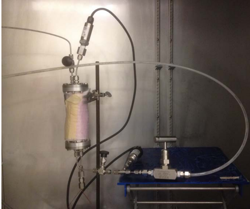
Figure 3. Chamber and related pressure and temperature sensors (X-ray transparent high-pressure sediment chamber inside of the environmental chamber)
