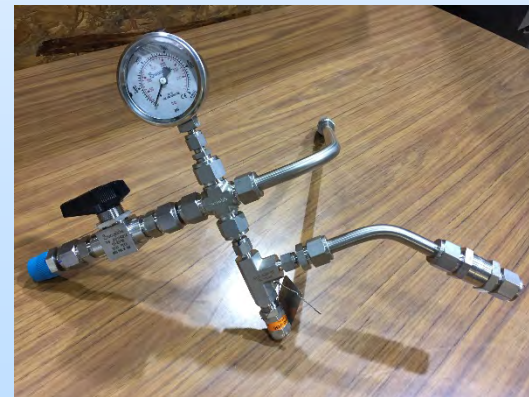
The Gage that Transfer Air Pressure to Fluid Pressure
