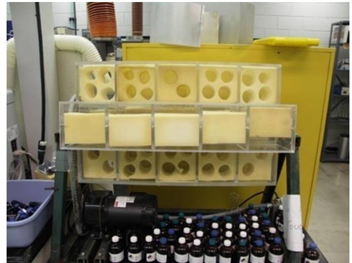
Rotating tumbler used for adsorption isotherm measurements at 23 \pm 1 °C
