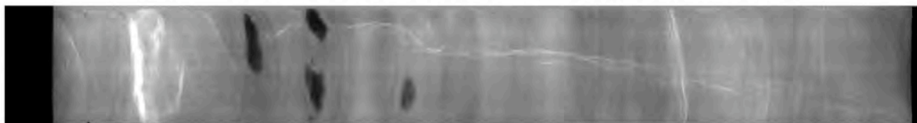
Core NGHP-1-21A-2Y 111 bar, 58.0 mbsf, gas hydrate veins, stored at pressure (SC-2)
