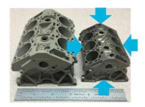
Powder bed method that uses polymer binder to hold layers together; results in fully dense part after sintering
