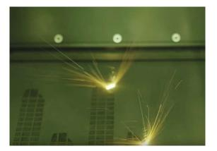
High-resolution laser sintering process; ideal for complex features and uncastable internal geometries
