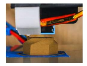
Metal-infused filament results in fully dense part after sintering
