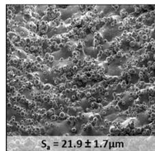
Additive manufacturing process parameters have promise in altering surface roughness.
