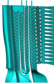
Cooled blade designs have been completed and now need to be manufactured
