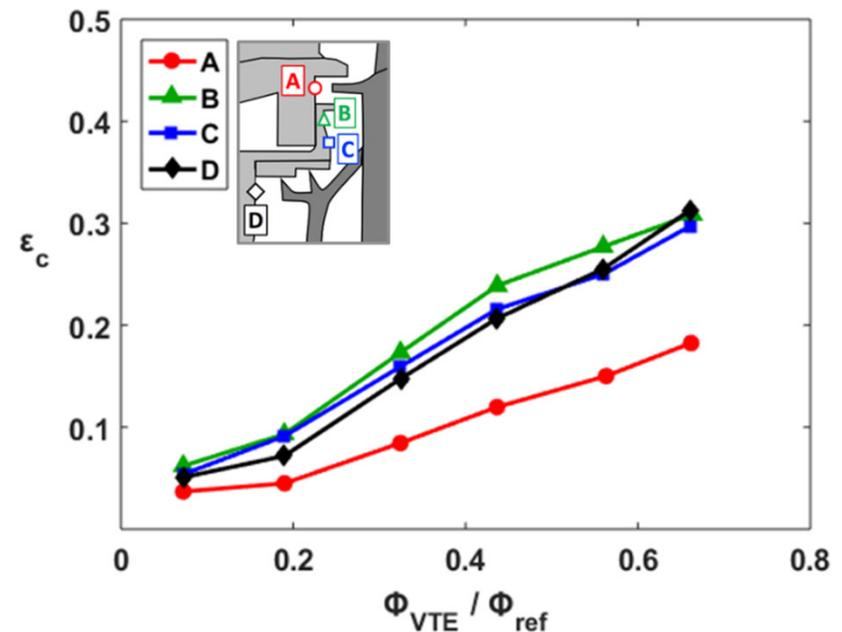
By holding the purge flow fixed while varying VTE flow, it was found that VTE influence in the wheelspace increased as VTE flow increased.
