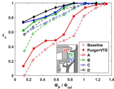
Vane Trailing Edge flow has a positive effect on the overall rim sealing effectiveness
