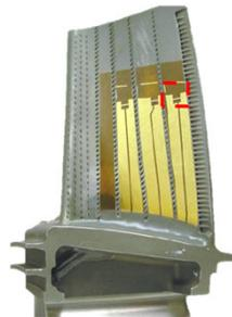
Heat flux gages for use in a steady facility have been evaluated.
