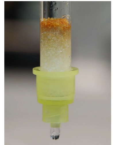
Capture of contaminants from water flowing through sorbent.
