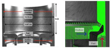
Fiure 2. Mesh of RDE facility at UM. Left: cross-sectional view, Right: injection scheme.
