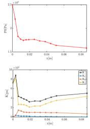
Figure 4. Axial total pressure, static pressure and kinetic energy x = 0 corresponds to the throat of the oxidizer injector.
