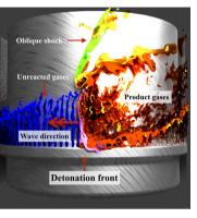
Figure 1. General detonation structure in numerical simulation of UM RDE
