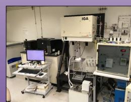
Hidden microbalance (IGA) used for gravimetric gas adsorption isotherm analysis.
