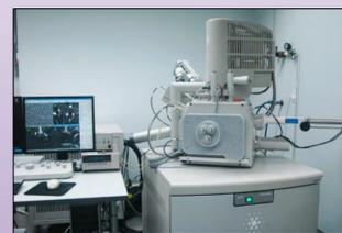
Scanning Electron Microscope used for feature relocation before and after dry/wet CO<sub>2</sub> exposure.
