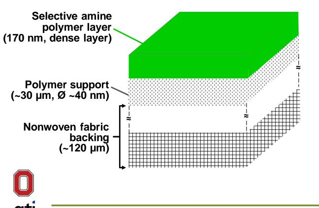
High-selectivity due to facilitated transport mechanism
