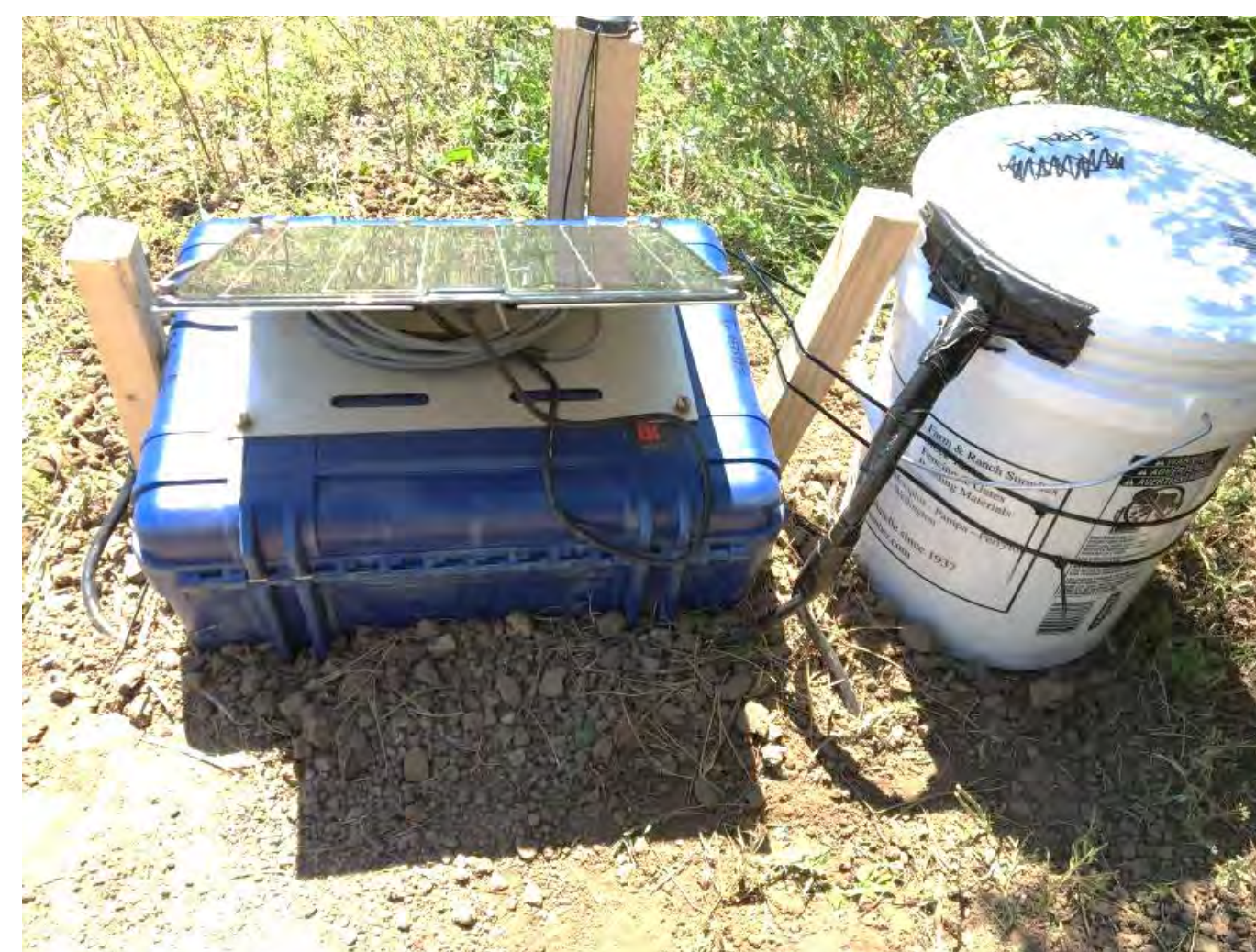
Figure 2. Example of a posthole seismometer station at the Farnsworth Site. Broadband seismometer sensor (right) is buried at about 1-m depth.
