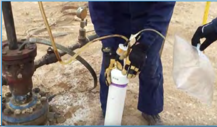
GOST: Gas Oil Separation Tank for collection of vapor-phase tracers
