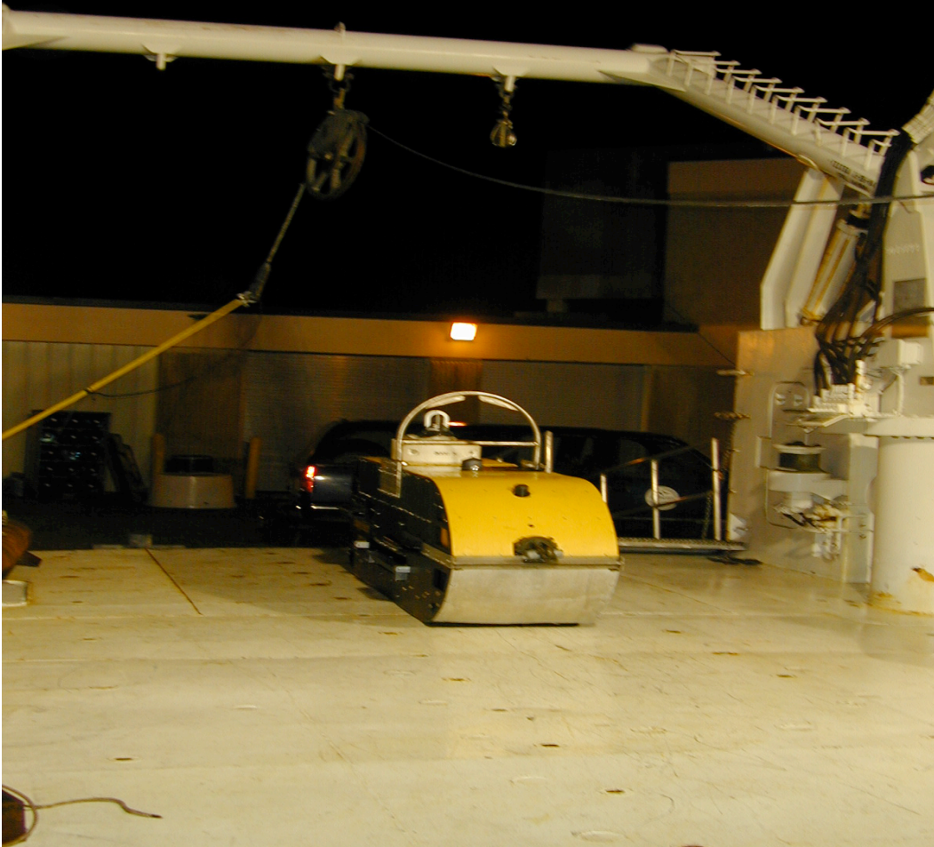
Figure 1. NRL's Deep-towed sidescan sonar, bathymetric and sub-bottom mapping instrument DT1.
