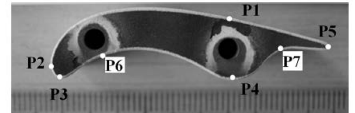
Fig. 1. Picture of a modified aerofoil-shaped specimen. P1, P2, P3, P4 and P5 are convex areas whereas P6 and P7 are concave.
