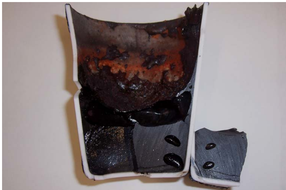
Figure 5.6: Cross-section of the slag glass melted in microwave low vacuum condition without using any susceptor. The “shiny” specs embedded in the glass are metallic particles (believed to be MAGNETIC iron)
