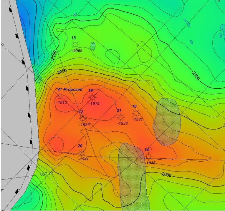
Figure 7. Map of East Barrow Gas Field with Proposed Hydrate Test Well Location
