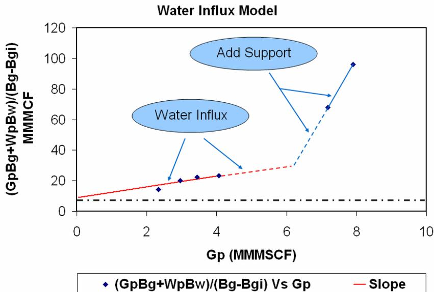
Figure 12. Water in Influx Model -  $(G_p B_g + W_p B_w) / (B_g - B_{gi})$  vs.  $G_p$  plot
