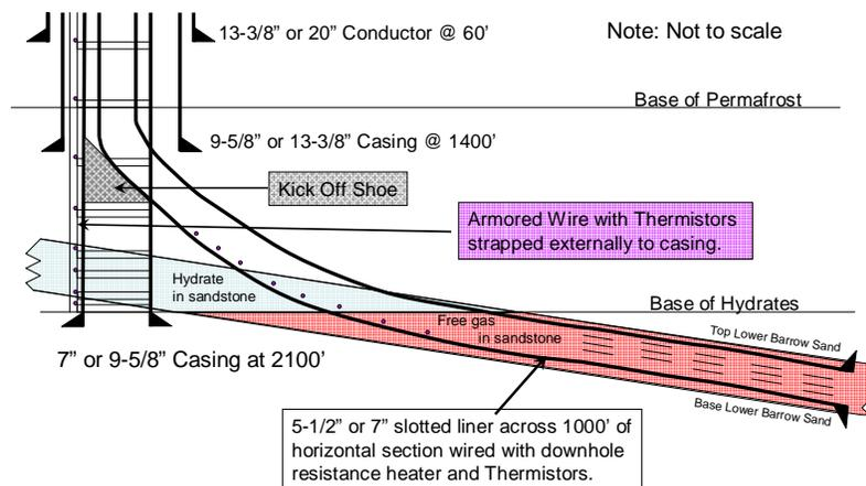
**Figure 18. Conceptual Hydrate Test Well Design**
