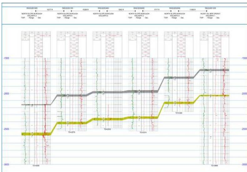
**Figure 2. Structural Well Cross-Section, SW-NE Through Walakpa Gas Field**
