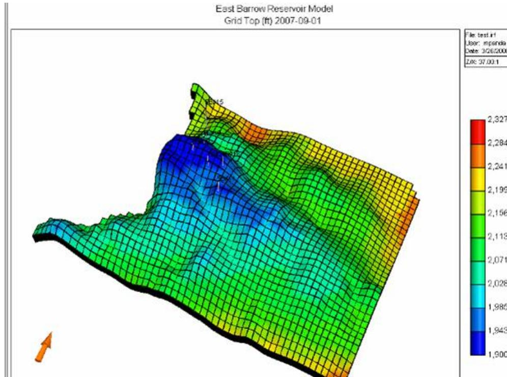
**Figure 3. Depth grid on Top Upper Barrow Sandstone, E Barrow Field**
