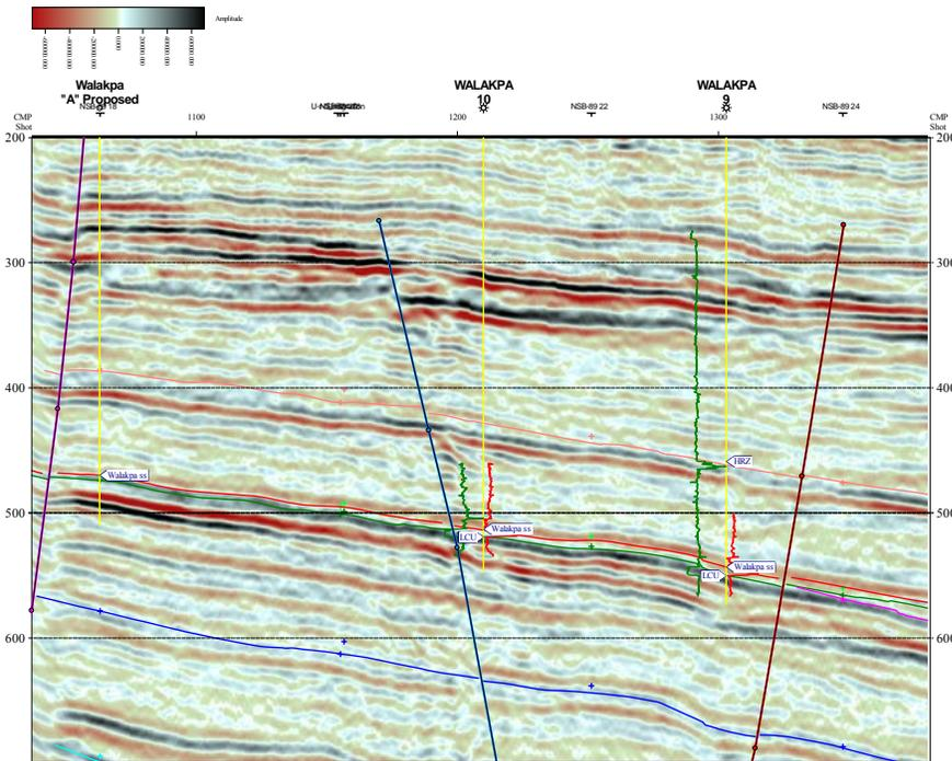
Figure 10. Seismic Line through Proposed Walakpa Hydrate Test Well Location
