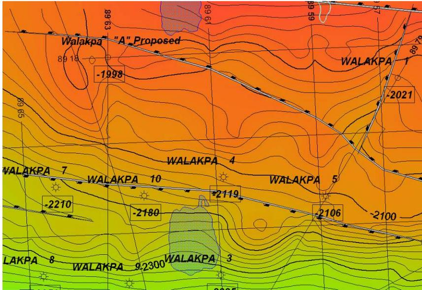
Figure 9. Map of Walakpa Gas Field with Proposed Hydrate Test Well Location
