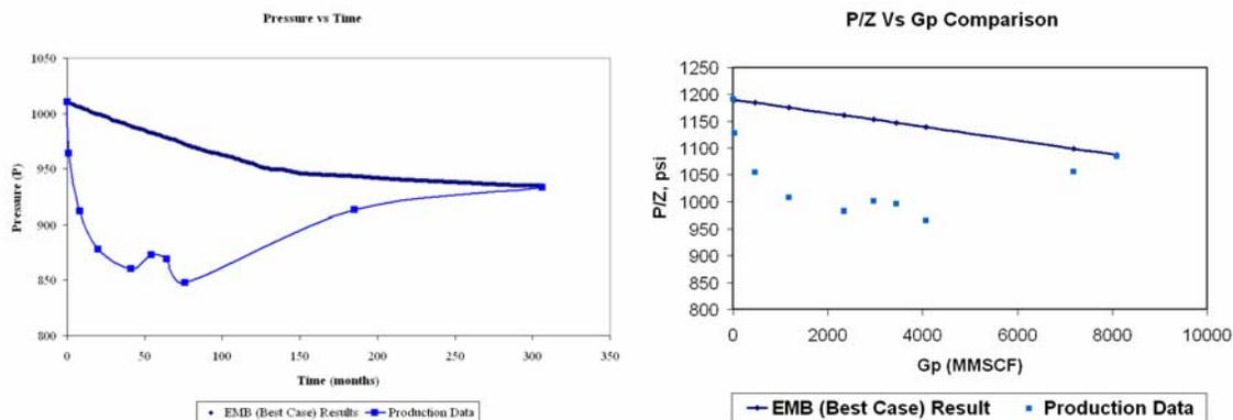
Figure 11. EMB Model – Pressure (P) vs. Time plot and P/Z vs.  $G_p$  plot for East Barrow gas reservoir
