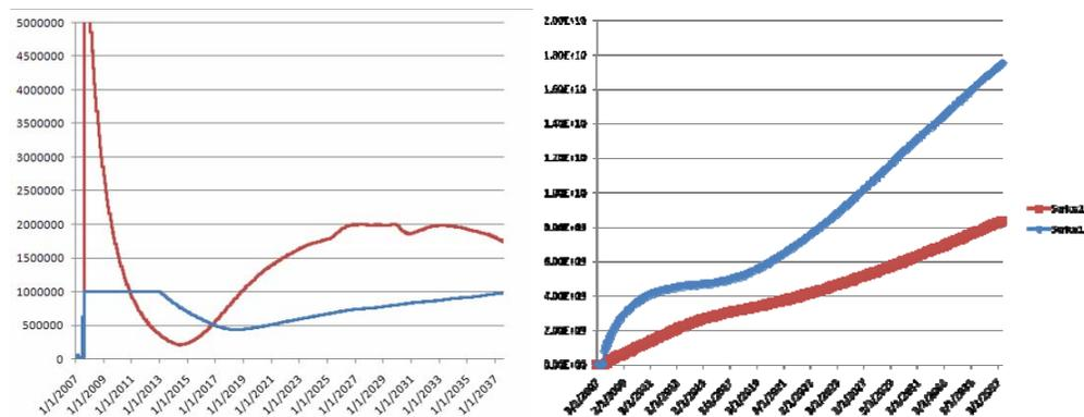
**Figure 17. Horizontal vs. Vertical Producer, Rate and Cumulative Gas Production, East Barrow (EB #14 Well)**
