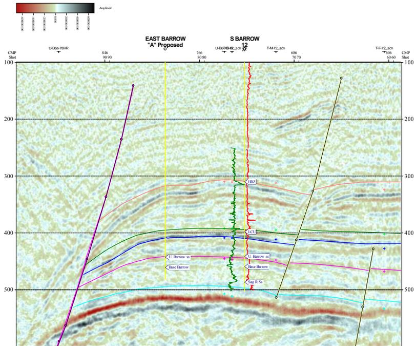
Figure 8. Seismic Line through Proposed East Barrow Hydrate Test Well Location
