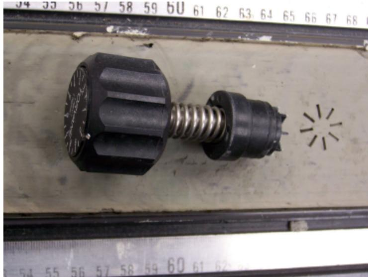
**Figure 13 – Torvane Shear Strength Device**
