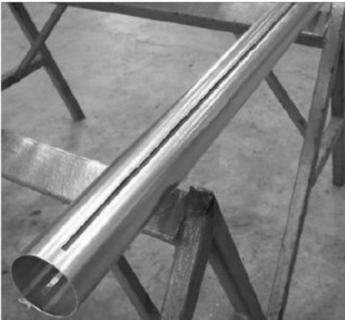
**Figure 7: Corion Inner Core Barrel with Slotted Liner**
