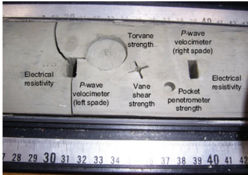
Figure 12 – Locations of Physical Property Measurements on Core Slab
