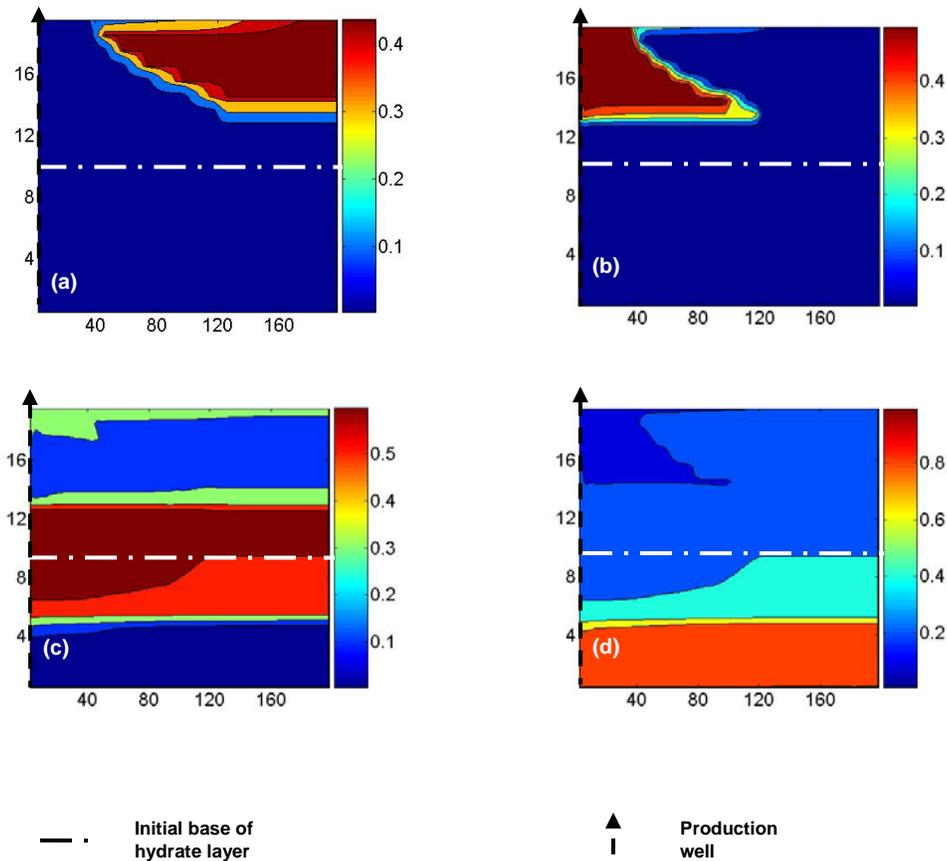
**Figure 2.** Contour plots of phase saturations at 1010 days after depressurization of a hydrate reservoir. The x-axis represents the horizontal distance from the production well, and the y-axis marks the vertical distance from the bottom of the reservoir. The scales of the coordinates are in meters: (a) Hydrate; (b) Ice; (c) Gas; (d) Aqueous phase [Sun & Mohanty, 2005].
