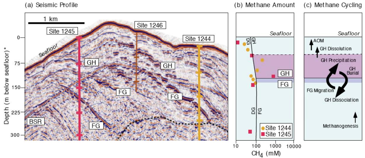
**Figure 1.** Seismic reflection profile across northern flank of southern Hydrate Ridge showing bottom simulating reflector (BSR) and drill site locations [Tréhu et al., 2003]. Also shown are in situ  $\text{CH}_4$  concentrations, depth zone of gas hydrate (GH), and inferred dynamic  $\text{CH}_4$  cycling.
