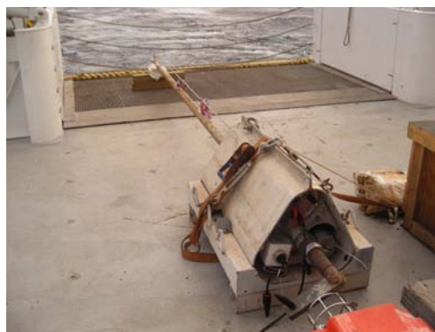
Figure 3: Lister-type heatflow probe.
